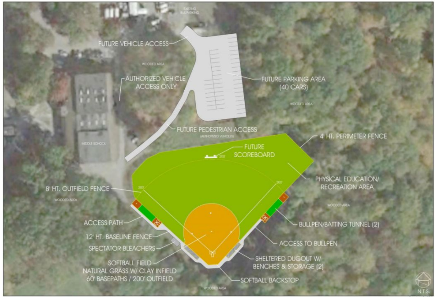
Schematic Plan- Softball Field Complex at Fox Lane Middle School Bedford Central School District SCALE: N.T.S.
